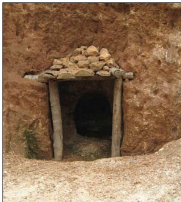
Entrance to a makeshift tunnel for digging cassiterite, on the road outside Lemera, South Kivu, August 2007.
